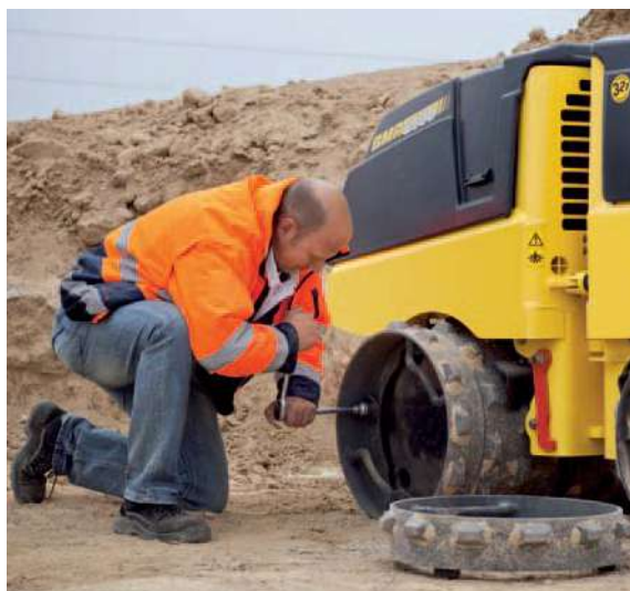
Optional drum extensions change the working width quickly to suit narrower or wider trench widths.
